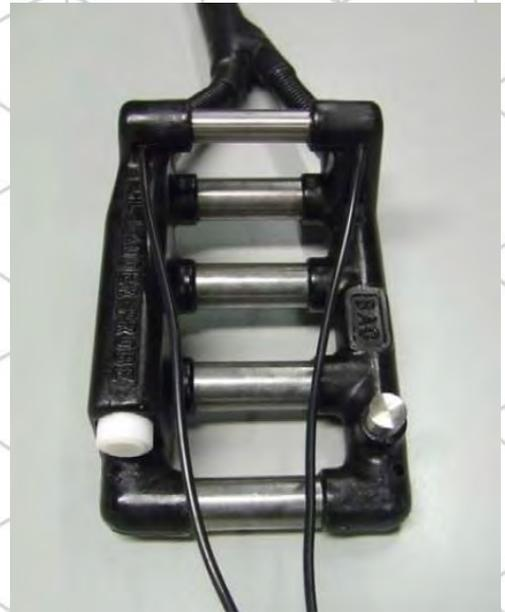
LPR Sensors for Corrosion Rate Monitoring
