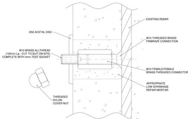
Figure 3 - Negative Connection Point - Pin Braze Type
