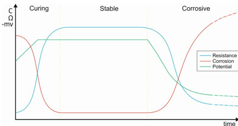
Figure 1 – Graph showing typical long term trends of steel in concrete corrosion. The above is a very simplified explanation of what generally happens and whilst use of the LPR equipment is relatively straightforward, the interpretation of the readings is not always so simple and this work should be carried out by a qualified person certified to at least level 2 (R Category) of the EN15257 standard or equivalent.
