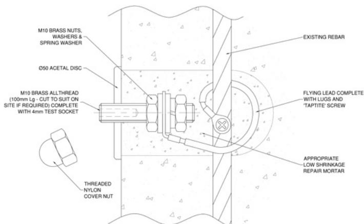
Figure 4 - Negative Connection Point - Taptite™ type
