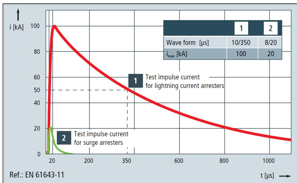
The diode and busbar assembly is designed to handle the above lightning strikes. In areas with high lightning activity we recommend fitting an **optional spark gap** co-ordinated to clamp and divert lightning strikes to ground without passing through the diodes and resistive busbar assembly thus reducing wear and increasing the life of the EDD.
