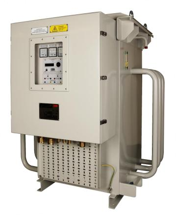
The transformer rectifier is built into an oil tank and control cabinet/s with the monitoring and control instruments mounted on an internally hinged control panel. The inner control panel includes a door interlocked isolator switch, providing electrical protection to the operator.
