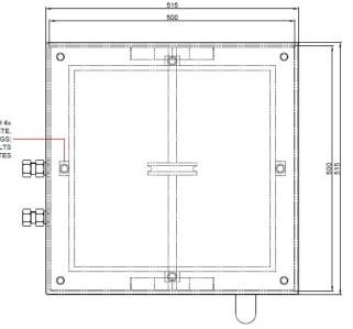
BASE HAS 50mm RETURN FLANGE WITH 4x 20mm HOLES FOR SECURING TO CONCRETE. KIT INCLUDES THE FOLLOWING FIXINGS: 4x M8 ANCHOR BOLTS
