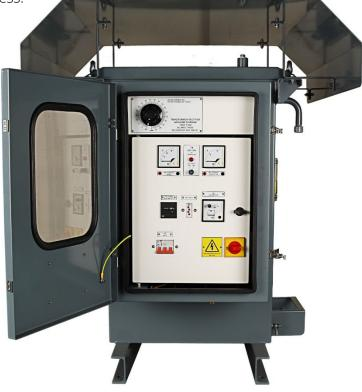
The transformer rectifier is built into an oil tank and control cabinet/s with the monitoring and control instruments mounted on an internally hinged control panel. The inner control panel includes a door interlocked isolator switch, providing electrical protection to the operator.
