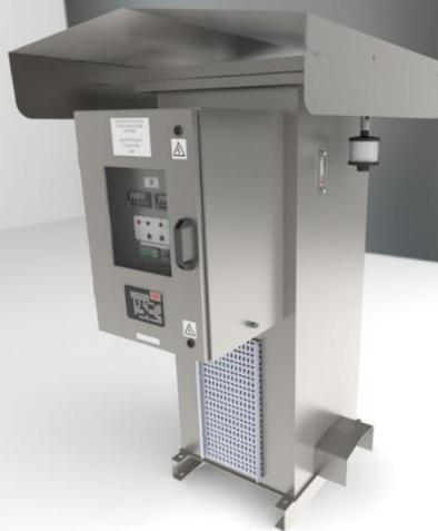
The transformer rectifier is housed inside an oil tank and control box with the control and indication mounted on an internal hinged door. The control box is fitted with a viewing window to enable easy viewing of the control and indication of the rectifier. The user is protected from High voltages via door interlocked isolator
