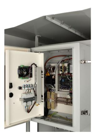
The transformer rectifier is built into an oil tank and control cabinet/s with the monitoring and control instruments mounted on an internally hinged control panel. The inner control panel includes a door interlocked isolator switch, providing electrical protection to the operator.
