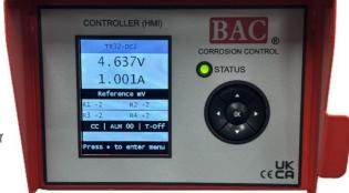
The HMI screen shuts down after 15 minutes of inactivity, for TR units with viewing window we include a wake button on the outside of the control cabinet to activate screen with opening the external door.
