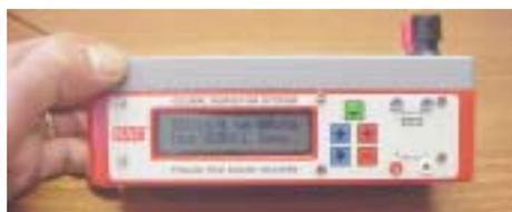
*The solid state unit is housed in a rugged IP65 sealed enclosure built to withstand a wide range of field conditions.*
