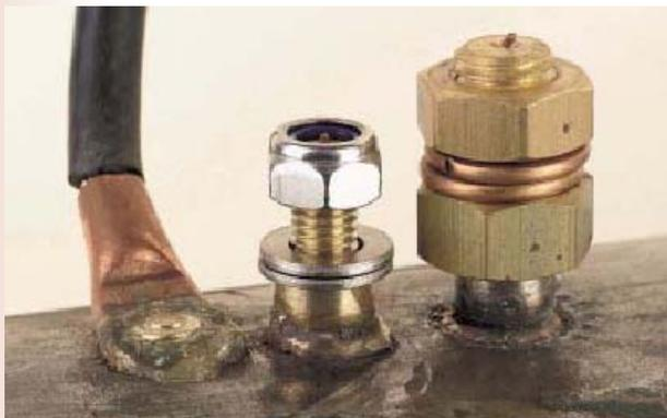
The Bright-Bond technique is safe, fast, durable and all weather. Due to its high mechanical strength, Bright-Bond Pin Brazing is an extremely effective and efficient form of electrical bonding.
