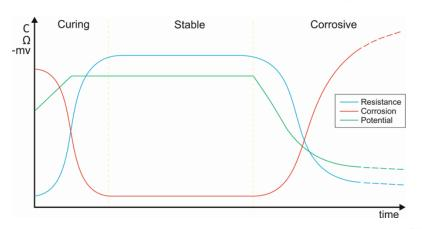
Figure 1 – Graph showing typical long term trends of steel in concrete corrosion The above is a very simplified explanation of what generally happens and whilst use of the LPR equipment is relatively straightforward, the interpretation of the readings is not always so simple and this work should be carried out by a qualified person certified to at least level 2 (R Category) of the EN15257 standard or equivalent.
