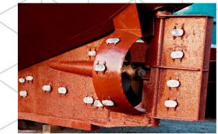
BAC offer a wide range pf Galvanic Anodes and Shaft Earthing systems for boats and ships.
