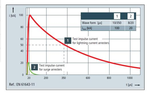
The diode and busbar assembly is designed to handle the above lightning strikes. In areas with high lightning activity we recommend fitting an **optional spark gap** co-ordinated to clamp and divert lightning strikes to ground without passing through the diodes and resistive busbar assembly thus reducing wear and increasing the life of the EDD.
